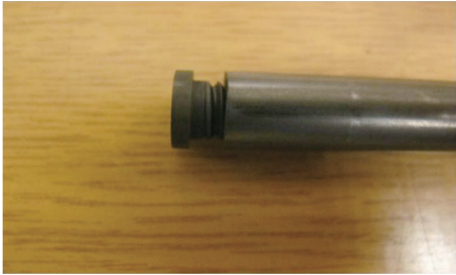
图 3 石墨基热电偶 Fig. 3 Measuring junction of graphite-based thermocouple
