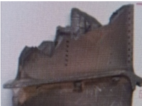
图 16 裂纹起源于气膜孔边缘的故障叶片 Fig. 16 Fault blade with the crack originated from the edge of the gas film hole
