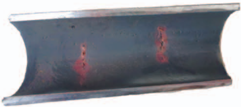
图4 换热管内表面 Fig.4 Inner surface of heat exchange tube
