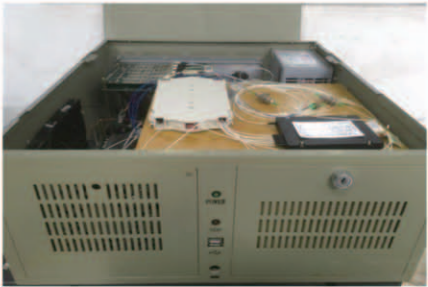
图 6 EFPI-FBG 光纤解调系统 Fig. 6 Demodulation system for EFPI-FBG composite optic fiber sensor
