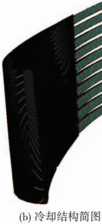
图 4 第一级导叶拓扑及内部冷却结构简图 Fig.4 Topology and simplified diagram of internal cooling structure for 1st stage guide vane
