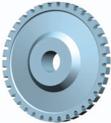
图2 涡轮盘典型结构 Fig.2 Typical structure of the turbine disk
