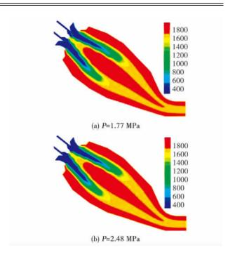
图 6 燃烧器中心截面温度分布/K Fig. 6 Temperature distribution in central cross section of combustor/K
